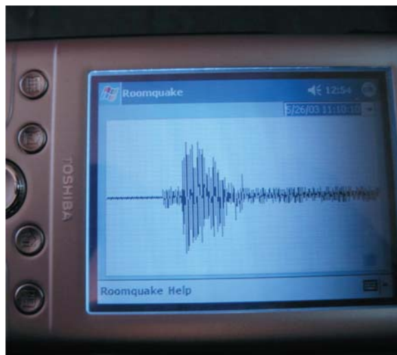
Figure 1. PocketPC serves as simulated seismograph.
