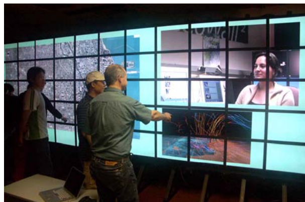
Figure 1: UIC's 100-Megapixel tiled display is managed by a software system called SAGE, which organizes the large-screen's "real estate" as if it were one continuous canvas [Jeong05], enabling researchers to view large-scale images while conducting high-definition video-teleconferences with remote colleagues.
